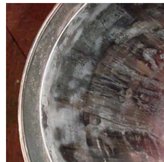
Man B&W 2-stroke cylinder liner damage from poor ignition quality.
